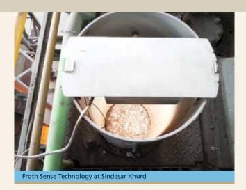
Froth Sense technology for Zn/Pb recovery improvement at Sindesar Khurd mine We have installed Froth Camera at Sindesar Khurd Mine. The Froth Sense technology is an advanced innovative image analysis technology for online measurement of flotation froth properties.
